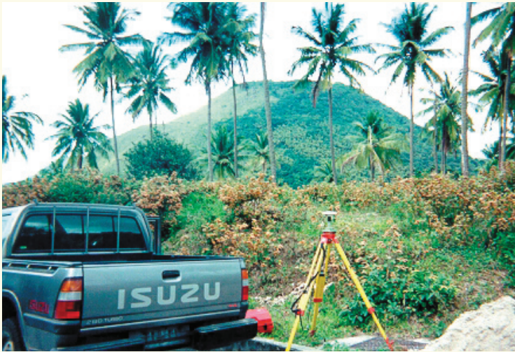
Ground deformation monitoring, near Terre Blanche, Soufrière Volcanic Centre
