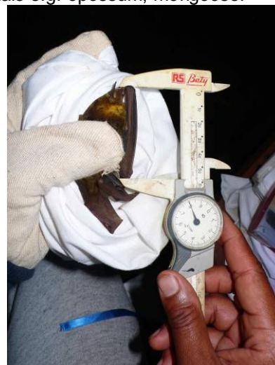
d) Using a calliper to measure the forearm length of a bat.
